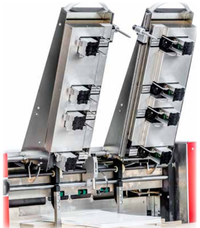
Sideblower arms swing up for access to loading bay
